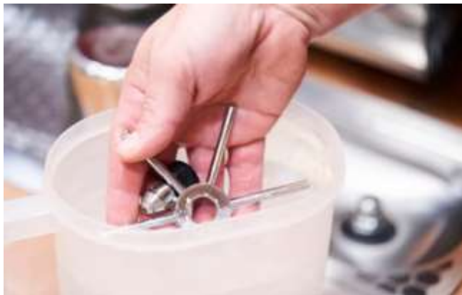
(A) Immerse the Spinjet and actuator star in the cleaning solution for 10 mins.
