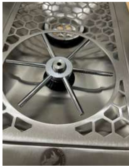
(B) While holding the actuator star in place, unscrew the Spinjet from the spray valve. (Be careful not to rotate or spin the actuator.)
