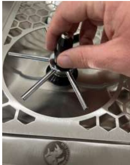
(B) Replace the wobble washer then spinjet by attaching it to the spray valve
