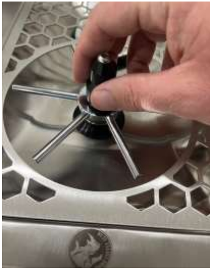
(A) Using an adjustable wrench, locate the 2 notches at the base of the spin jet
