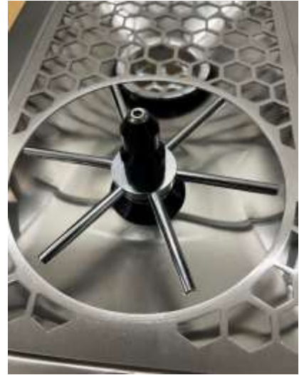
(C) Tighten with an adjustable wrench & replace the drain tray.
