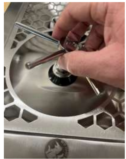
(C) Remove the actuator star by lifting it over the top of the valve
