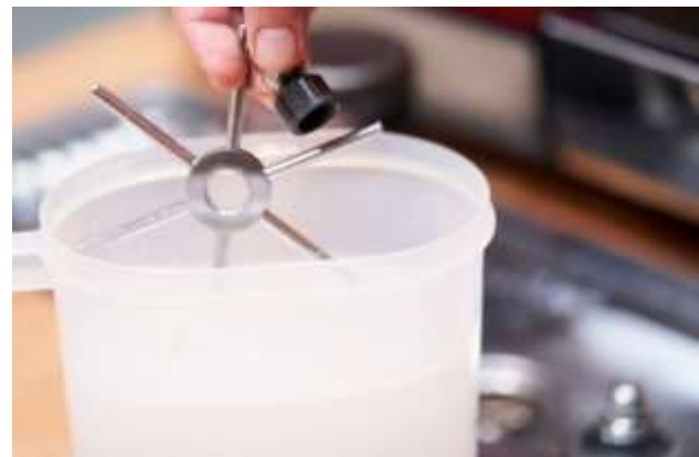
(A) Immerse the Spinjet and actuator star in the cleaning solution for 10 mins.
