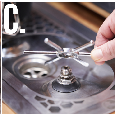
(C) Remove the actuator star by lifting it over the top of the valve
